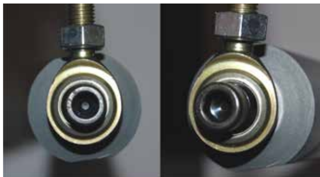
Figure 44. Heim Joint Orientation
